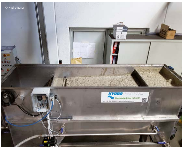
The new oil separator.
